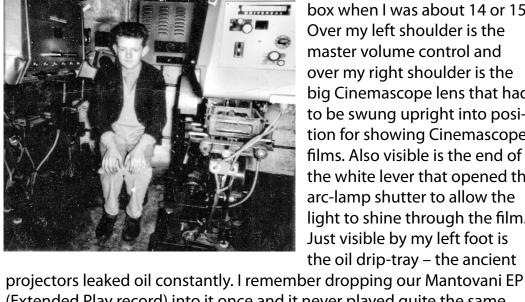
box when I was about 14 or 15. Over my left shoulder is the master volume control and over my right shoulder is the big Cinemascope lens that had to be swung upright into position for showing Cinemascope films. Also visible is the end of the white lever that opened the arc-lamp shutter to allow the light to shine through the film. Just visible by my left foot is the oil drip-tray – the ancient (Extended Play record) into it once and it never played quite the same
